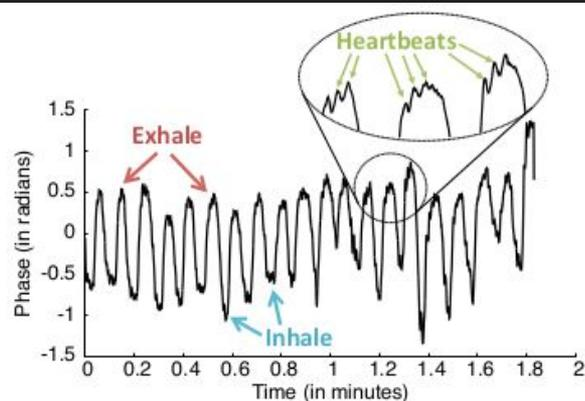
**Figure 3—Phase variation due to vital signs.** The figure shows the variations in phase due to breathing and heartbeats, where peaks and valleys in the phase correspond to exhale and inhale motions respectively; also, zooming in on the signal allows us to observe the heartbeats modulated on top of the breathing motion.
