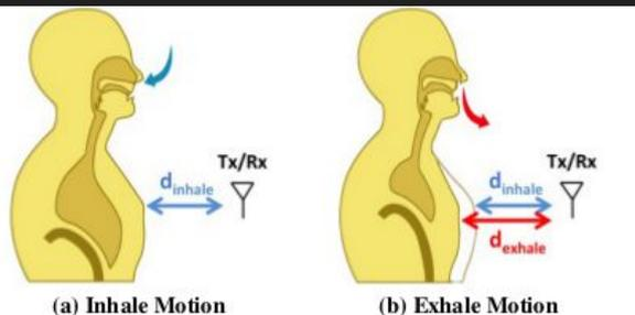
**Figure 1—Chest Motion Changes the Signal Reflection Time.** (a) shows that when the person inhales, his chest expands and becomes closer to the antenna, hence decreasing the time it takes the signal to reflect back to the device. (b) shows that when the person exhales, his chest contracts and moves away from the antenna, hence the distance between the chest and the antenna increases, causing an increase in the reflection time.
