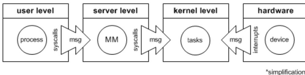
For a process to make a system call, it must send a message to the server level. Specifically, a user process must send a message to either MM or FS. The servers may then send any necessary messages to the kernel level.
