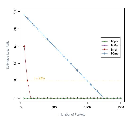
Figure 3.11: The effect of packet size and path capacity on detectability in the simulated environment ( $c_p = 1$ Mbps).
