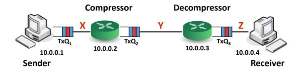
Figure 4.4: Topology used for simulations in the presence of compression link on the path is complete.  $\hfill \Box$
