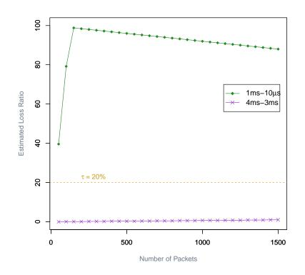
Figure 3.6: Detectability between scenarios ( $\delta_i = 1\mu$ s and  $\delta_i = 1$ ms) vs. ( $\delta_i = 3$ ms and  $\delta_i = 4$ ms) in the simulated environment ( $\ell = 100, c_p = 100$ Mbps).
