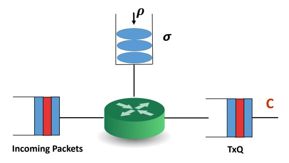
Figure 6.1: How traffic shaping works (token leaky bucket algorithm)
