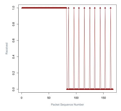
Figure 3.7: Observed loss pattern after queue saturation in the simulated environment  $(\ell = 100, c_p = 100 \text{Mbps}).$
