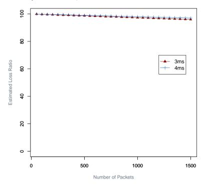
Figure 3.5: Loss ratio difference between when  $\delta_i = 3$ ms and  $\delta_i = 4$ ms in the simulated environment ( $\ell = 100, c_p = 100$ Mbps).
