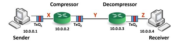
Figure A.3: Simple topology to test our implemented LZ compression module.
