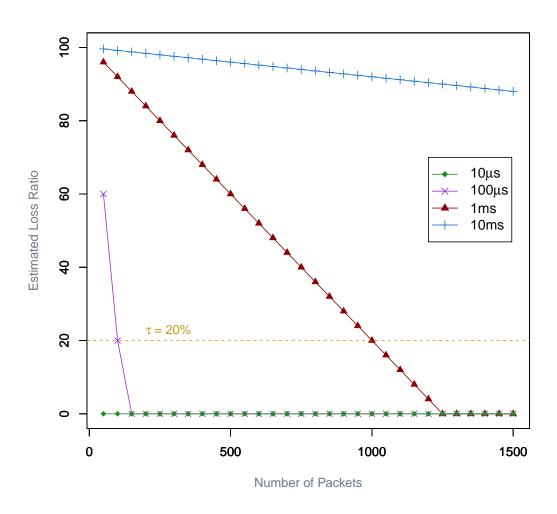
Figure 3.10: The effect of packet size and path capacity on detectability in the simulated environment ( $c_p = 10$ Mbps).
