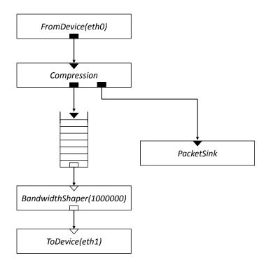
Figure A.8: Click configuration file tree diagram to use the LZ compression element.
