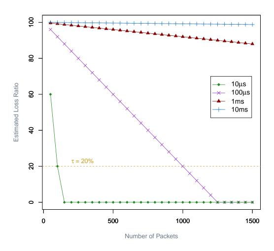
Figure 3.9: The effect of packet size and path capacity on detectability in the simulated environment ( $c_p = 100$ Mbps).
