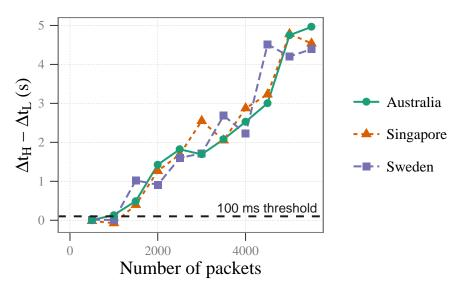
Figure 7.6: Comparison of the number of probe packets used for detection when using only a single measurement from three geographically diverse distant PlanetLab nodes.
