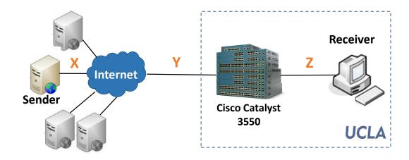
Figure 5.5: Environment used in our Internet experiment with the help of contributors to throttle the last link (Z = 100Mbps).
