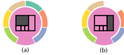
Fig. 2: The history glyph which help users navigate states on the blockchain. In (a) all seven collaborators were present when a change was made to the top left panel (dark gray highlight) while in (b) one collaborators was absent (green segment) when a change was made in the panel on the right (dark gray highlight).
