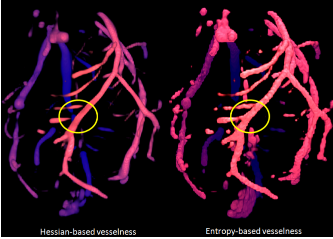
Fig. 4. Visualization using polar profile compared to visualization using Hessian techniques. The regions marked with a yellow circle clearly show that our technique performs better at branch points.
