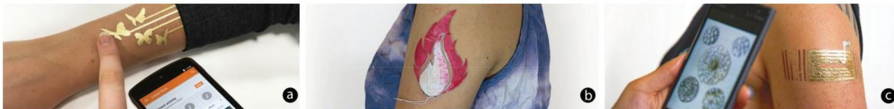
**Figure 1: DuoSkin is a rapid prototyping and fabrication process using the skin-friendly material gold leaf to create wearable on-skin user interfaces, such as (a) sensing touch input, (b) displaying the user's mood using a thermochromic tattoo, and (c) communicating and sharing data with other devices through NFC—all while maintaining body decoration aesthetics.**
