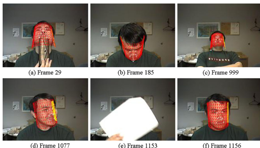
Fig. 19.3 Example of 3D head tracking, including re-registration after losing the head
