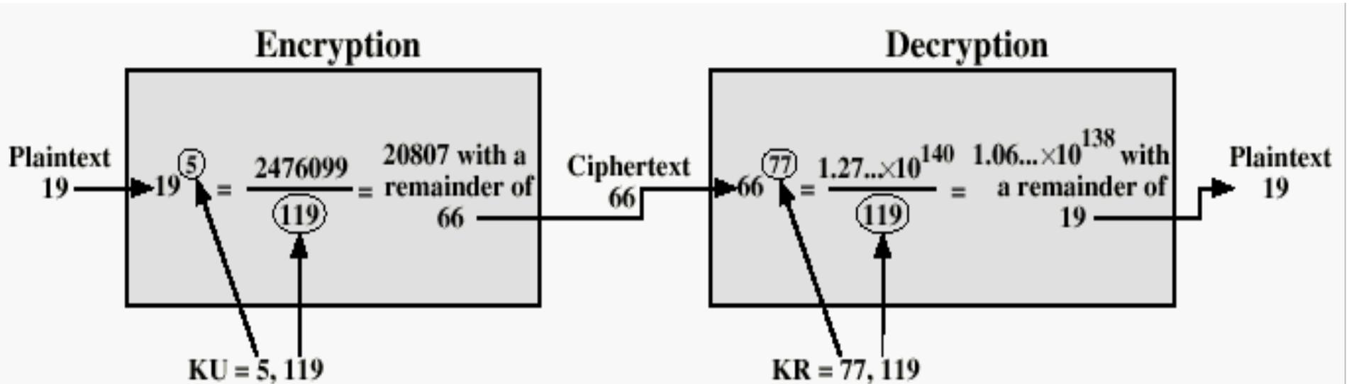
Figure 3.9 Example of RSA Algorithm
