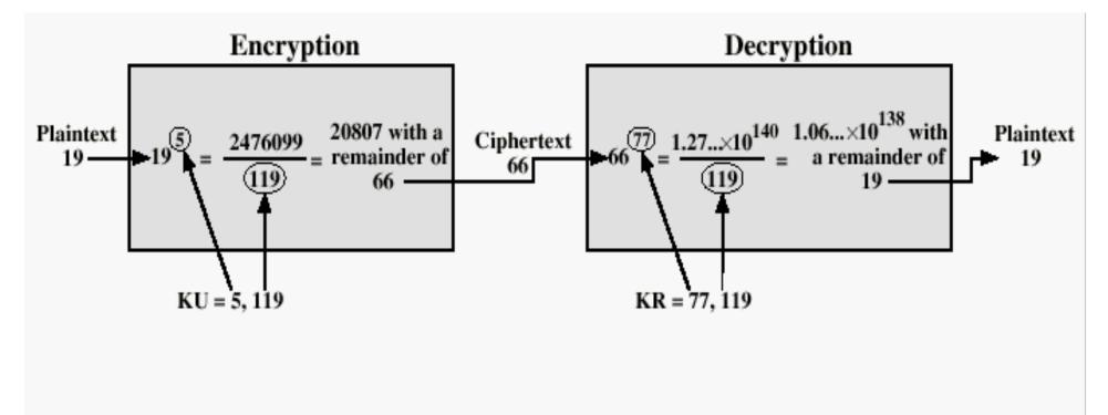
Figure 3.9 Example of RSA Algorithm
