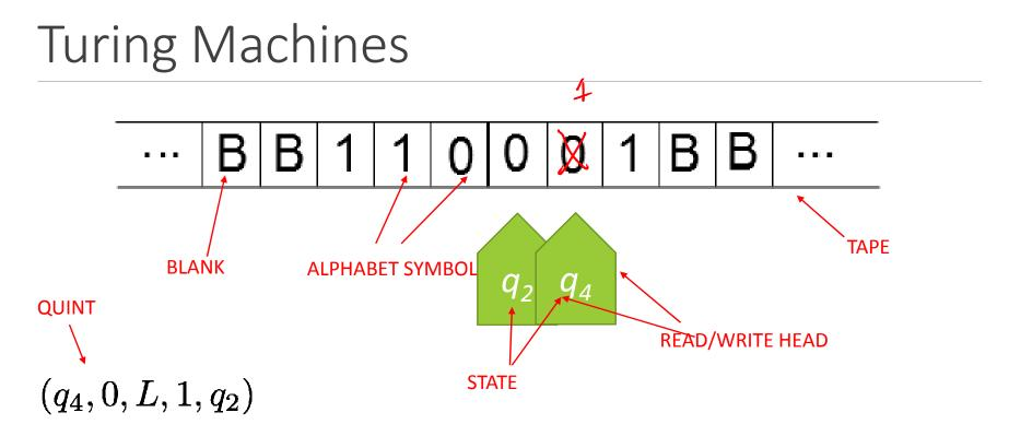
For the TM, the quint is an instruction: If I am in state  $q_4$  reading symbol 0, I will write symbol 1 into the cell, change my state to  $q_2$ , and make move L.
