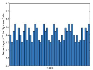
Fig. 2. Distribution of files in the system using our two-tiered hierarchical hashing scheme.
