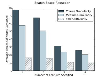
Fig. 3. Reduction of the search space with different tick mark configurations as more dimensions are added.
