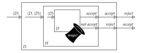
However, when we do this we get a contradiction (in red). The outer D must reject when the inner D accepts. A Turing machine cannot both accept and reject at the same time on the same input. Therefore, H must not exist.
