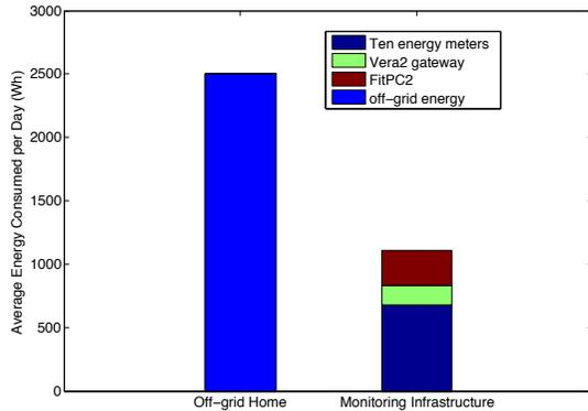
**Figure 2.** The figure illustrates the energy overhead of our monitoring system compared to the per day energy consumption of an off-grid home.
